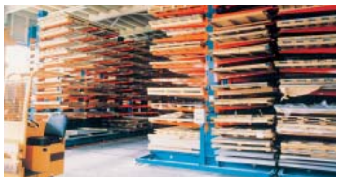
Mobile metal sheet storage
